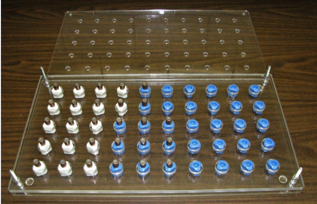
Figure 7: Plexiglass jig used for epoxying bullets to plastic mounts. The cover plate (not attached) is shown above the base that holds the plastic mounts. The left half of the jig has bullets already epoxyed to the mounts, for illustrative purposes.
