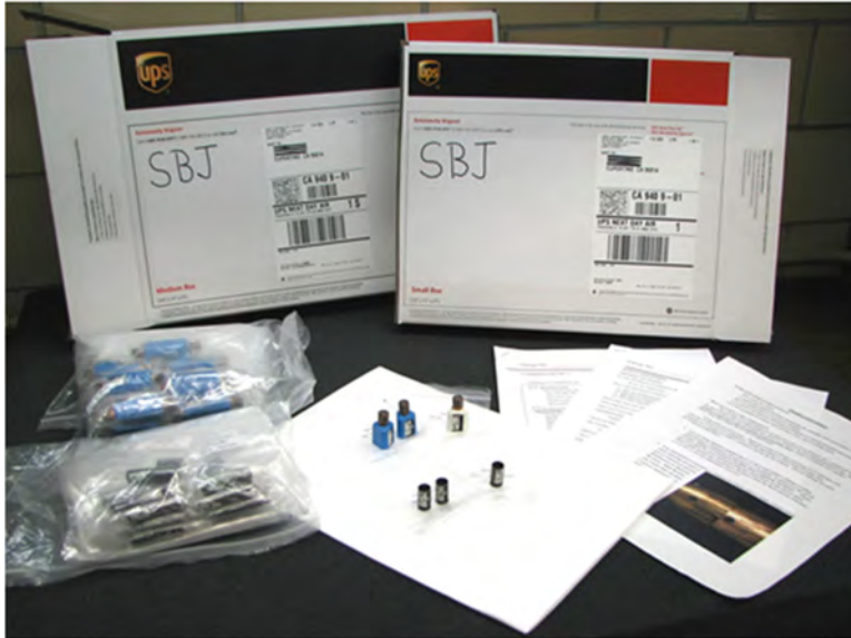
Figure 9: Sample packet components, including the bullet and cartridge case test sets, forms, and shipping and return boxes.
